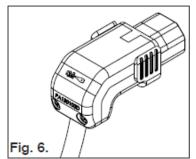
Replace the cord grip (Fig. 4 & 5.) ensuring the torque value is achieved (0.3Nm), and then replace the outer housing and screws (Fig. 6.).
