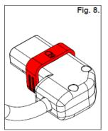
Replace the cord grip (Fig. 7.) ensuring the torque value is achieved (0.3Nm), and then replace the outer housing, screws and handle (Fig. 8.).
